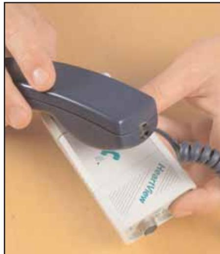
Figure 3. Acoustic transmission of ECG via phone
